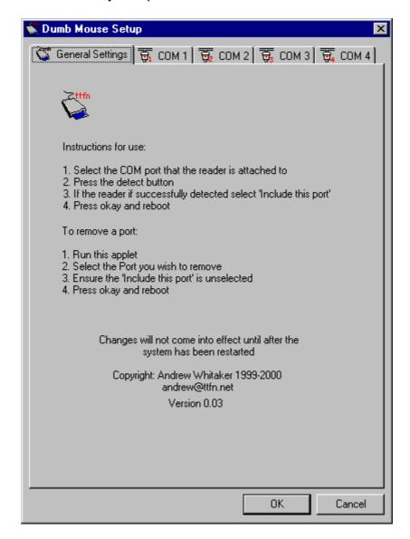
Select the COM port that your reader is attached to. In the following example the reader is attached to COM 1.
