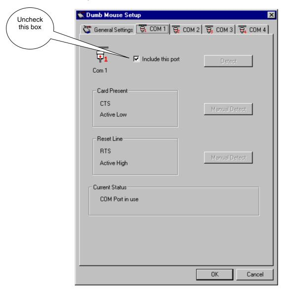
Uncheck the "Include this port" box and press OK. At this point you will either need to stop the appropriate services (Windows NT/2000) or reboot the computer (Windows 95/98).
